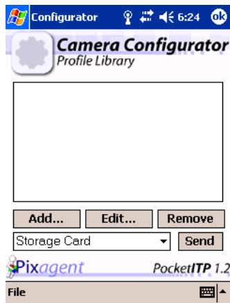
Figure 6.1: The main configurator window allows you to manage a library of profiles for various venues. Using this list you can manipulate your profiles as well as prepare memory cards to load the settings into your camera.
