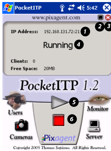
Figure 7.1: Description of the main window controls: (1) The IP Address and socket that the server is running on, (2) The LCD-off button, (3) The exit button, (4) The server status indicator, (5) The start button, (6) The stop button.
