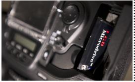
Remove the CF card from your computer and insert it into the camera with the WT-1 attached. Wait: for the green light to go out, then press the *Menu*: button. Navigate to the Set Up tab (the bottom tab): and continue on to the next step...
