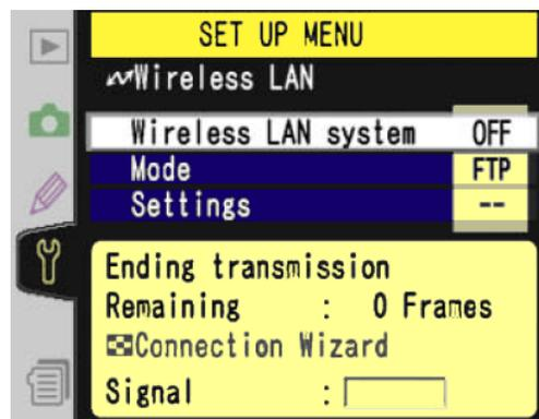
Once the *Wireless LAN* menu appears select the *Wireless LAN system* entry and switch it to the *OFF* position.
