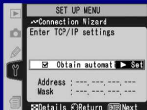
After the camera has connected to the appropriate wireless network, the next step is to specify the TCP/IP properties. If the fields aren't already set, use the values specified in the green section of the Control Centre.
