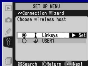
Once the connection wizard is started, it will first show you a list of available wireless networks. Select the appropriate network and then press the Enter button to move on to the next step. If the selected network uses encryption, you may be prompted for additional information.
