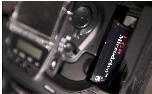
Remove the CF card from your computer and insert it into the camera with the WT-2 attached. Wait for the green light to go out, then press the *Menu* button. Navigate to the *Set Up* tab (the bottom tab) and continue on to the next step...
