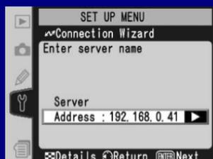
The next step in the wizard prompts you to specify the server that you would like the images transmitted to. The *IP Address* value in the red section of the Control Centre should be entered at this stage. Press the enter button to commit the selection and move on.
