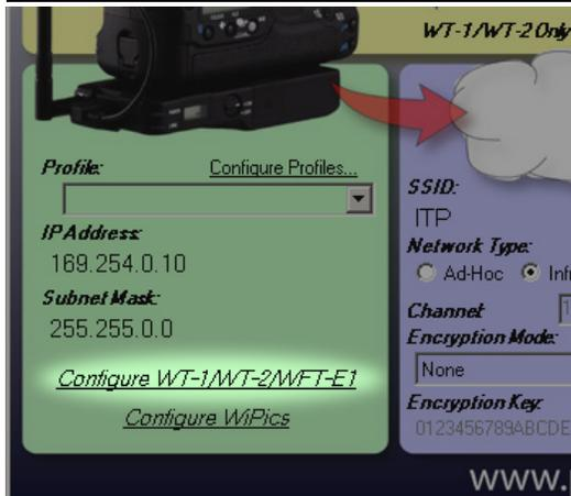
Once the specified settings have been selected, click the *Configure WT-1/WT-2/WFT-E1* link to begin the process of configuring your camera. Follow the provided directions to load these settings onto a memory card.
