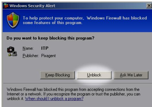
If the Windows Firewall is enabled on your computer, you will be prompted to continue blocking ITP. When this dialog pops up, select the *Unblock* button to allow ITP to receive connections from the camera. This is necessary for proper operation of your system.
