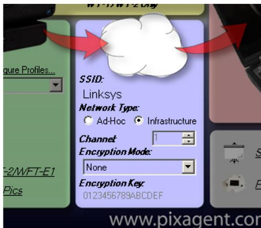
Once the *Control Centre* interface comes up, enter the wireless settings that you are currently using in the blue section. Please refer to the settings used in your access point/router for the correct values.
