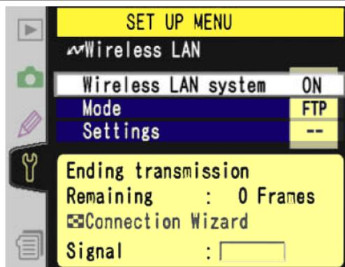
When the settings have been loaded, return to the *Wireless LAN* menu. Return to the *Wireless LAN system* entry and switch it back to *ON*.
